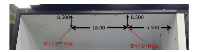
4. Install pop rivets and assembly mounting clips in drilled holes in direction as shown below and use pop rivet gun to fasten to top of cabinet.
